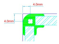
Dimensions for location of drilled holes, for fixing of PETG plastic end caps.
